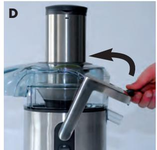
**Important:** If the safety locking arm is not in the right position the motor will not start moving and the display shows "Lockbar".
